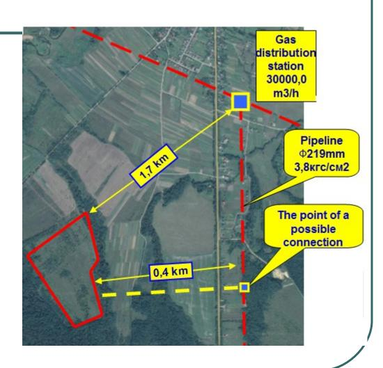
Capacity margin of the gas distribution station - 30000,0 m3/h
